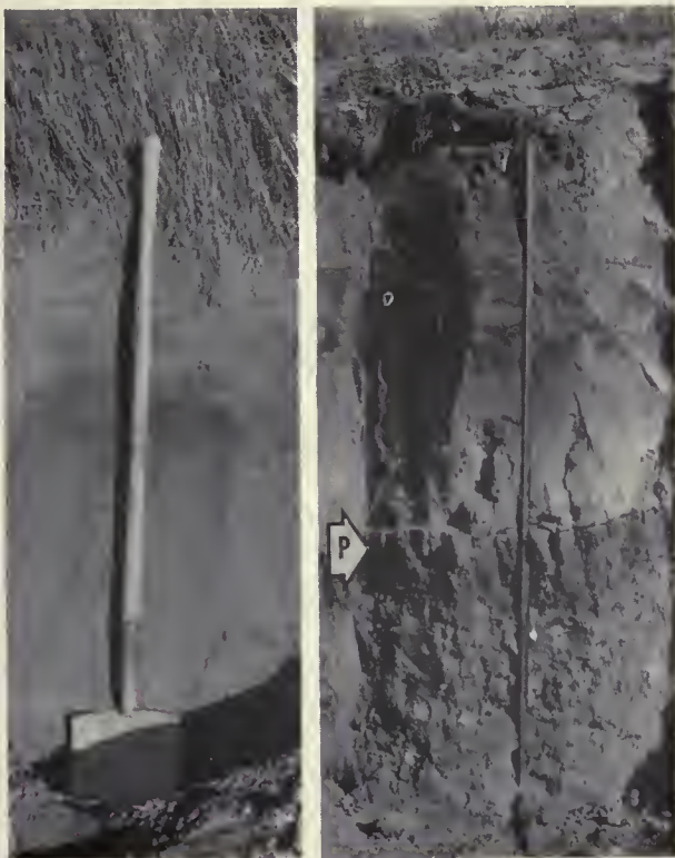
THE SOIL'S THE THING which in a large measure determines the success of a Federal Reclamation project. At left, a deep, permeable, fertile soil, well suited to irrigation. At right, a soil with a clay-pan layer (P) at a depth of 27 inches—not well suited to irrigation. Photos by Phil Merritt, Region 1 photographer.
